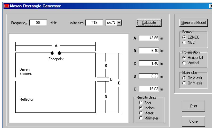
For this loop, using the numbers above, the driven element is two lengths of wire, each  $(43.69/2 + 6.40 =) 28.25$  inches, while the reflector is a single piece of wire that is  $(43.69 + 8.23 + 8.23 =) 60.15$  inches. I used 18 gauge stranded speaker, which has a soft plastic jacket which doesn't kink.
