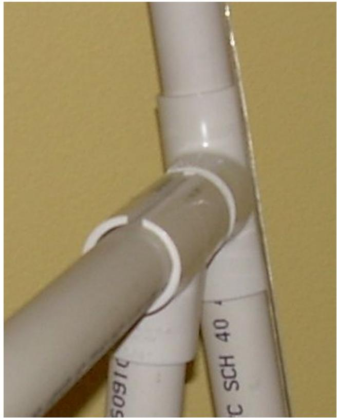
**Close-up of pivot tee connector assembly**
