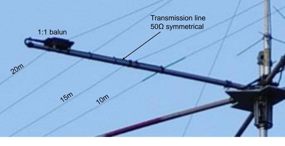
The three dipoles are connected to the parallel transmission line, fed by the balun.
