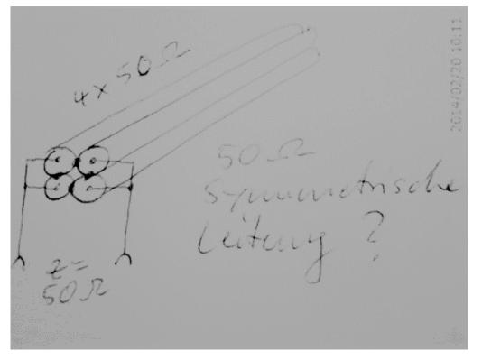
The 50  $\Omega$  transmission line is made out of two pairs standard 50  $\Omega$  Coax Cable. Do **not** use standard symmetric cable with some hundred  $\Omega$  impedance. This will end up in unwanted transformation and in detuned Moxon, unexpected directivity included. I`ve been down to this road  $\odot$
