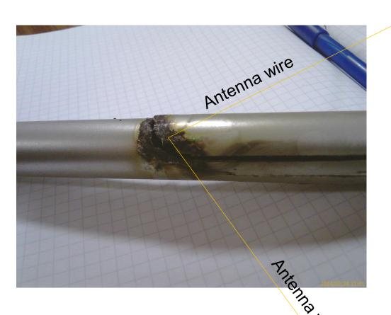
...followed by a mechanical failure of one fibre rod...
